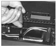
Figure 21: Orifice Removal.
